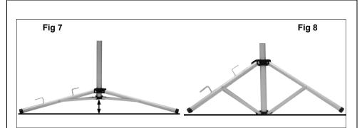
IMPORTANT: Ensure the legs are spread wide enough so that the centre column is clear of the ground as shown in Fig 7., otherwise the centre column will act as a fourth leg and the stand will therefore be unstable. Fig. 8 illustrates the stand in an unstable condition.
